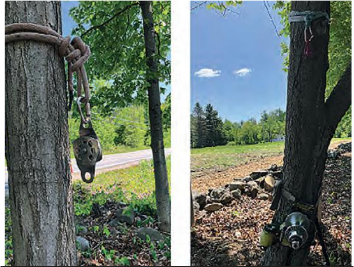
Photos 8 and 9 : The lowering line ran down to an adjacent rescue pulley on a nearby maple tree (left), then to another small redirect fairlead pulley, which guided the lowering line into our Hobbs H2 Lowering & Lifting Device (LD) mounted on another sturdy maple tree (right).
