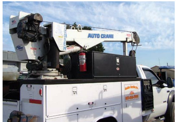
Fig. 2. The rotating pedestal-mounted service truck boom simplifies lifting.
