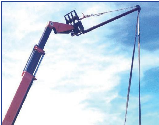
Fig. 1. Shop-made, all-terrain hoist. Who was the design engineer?
