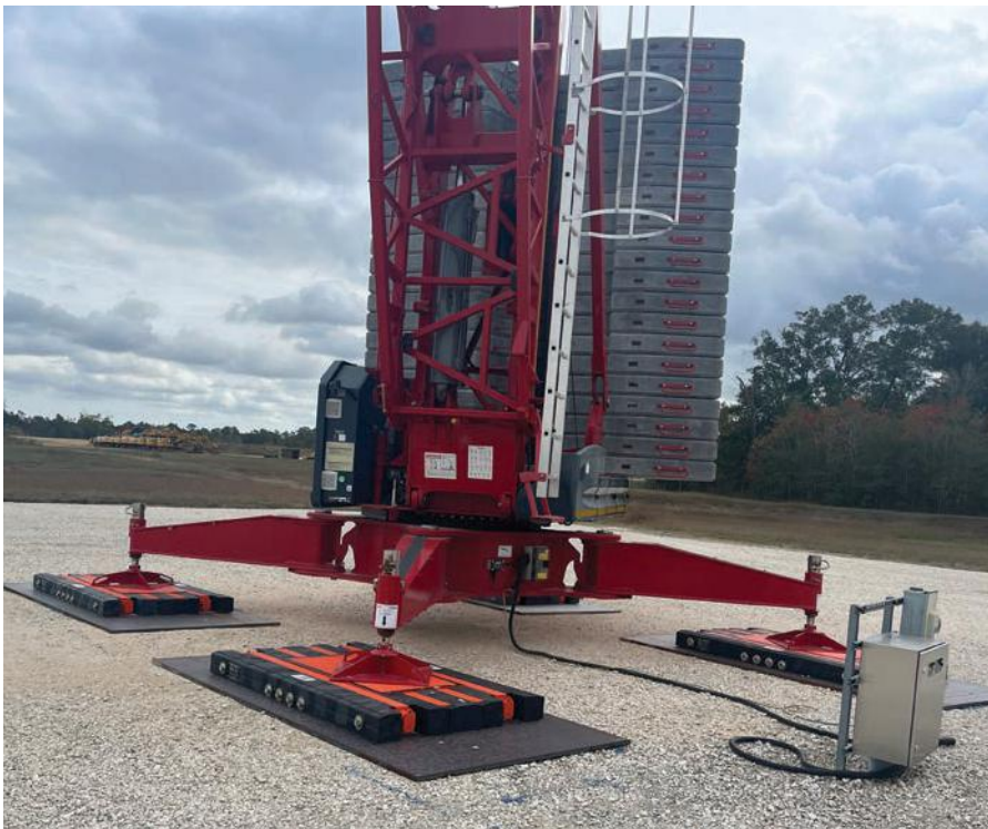
The IUOE training center's new Potain IGO T99 self-erecting tower crane set up on DICA EcoMax crane pads.
