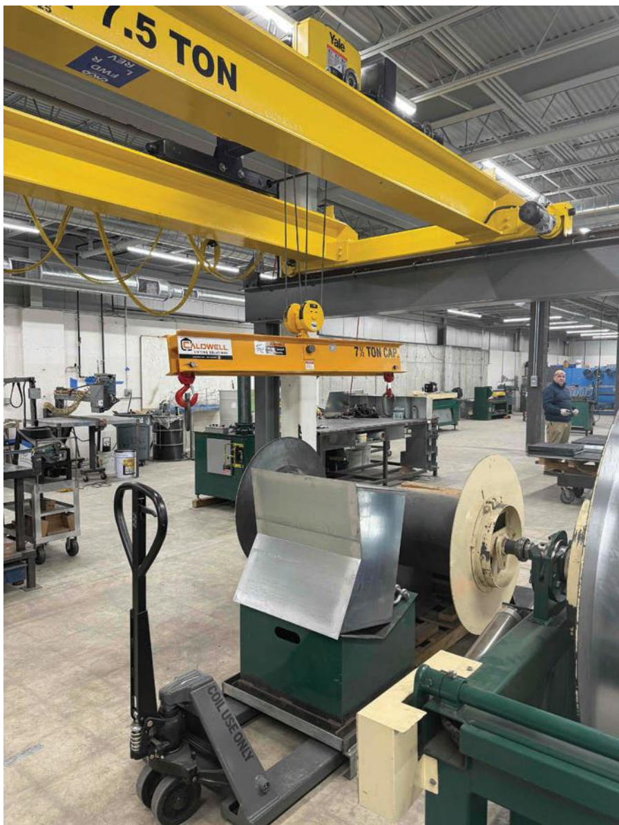
The Caldwell Group engineered a 7.5-ton capacity, low-headroom multiple spread lifting beam for handling steel coils with greater safety and precision. When vertical space is limited, solutions like Caldwell’s Model 20 multiple spread lifting beam don’t just improve workflow, they reduce risk.
