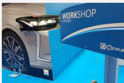
Advanced AFS function: enables AFS headlights to be set, calibrated and configured.
