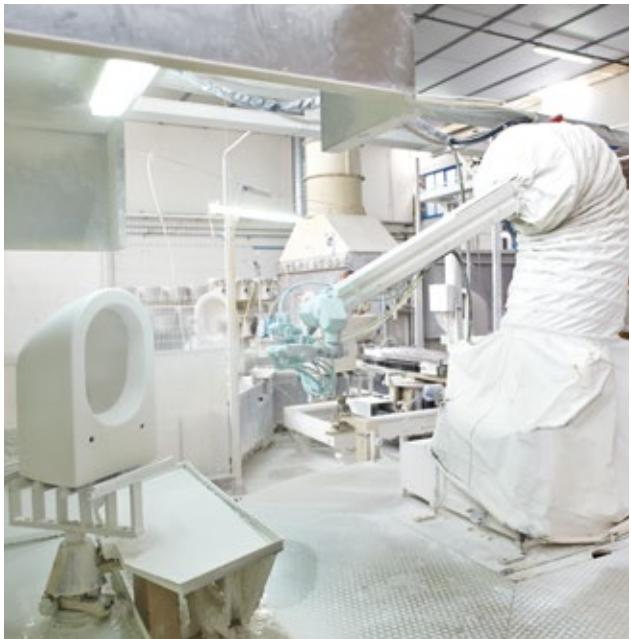
Automation of the movement of the pieces makes for an orderly transition from one phase to another while constantly ensuring the object's safety. Once the initial glazing is over, the piece goes on to the second glazing. After around 15 minutes it is ready for baking.
