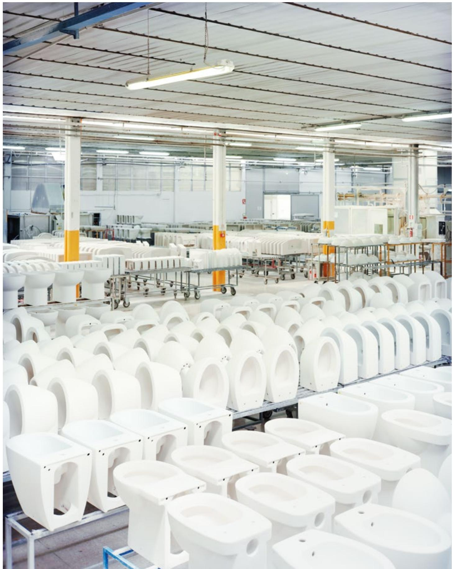
After the glazing process, the pieces are put on trolleys and sent for firing. The order in which the mobile trolleys are filled necessarily follows the sequence realized during the glazing phase. This order will later be changed for access to the kiln.
