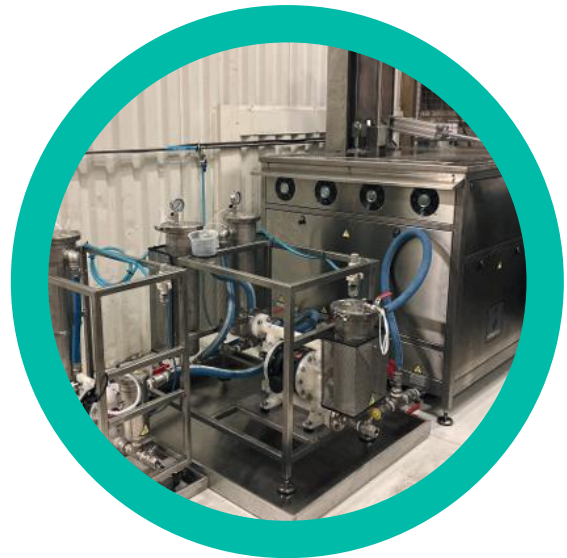
Ultra-sonic cleaning (solvent-free) machine, Nantes
