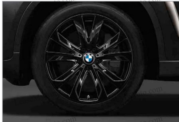
Star Spoke High-gloss Black light alloy wheels (Style 491) 20 x 10.0 front, 20 x 11.0 rear; and 275/40 front, 315/35 rear run-flat performance tires 1,2,3
