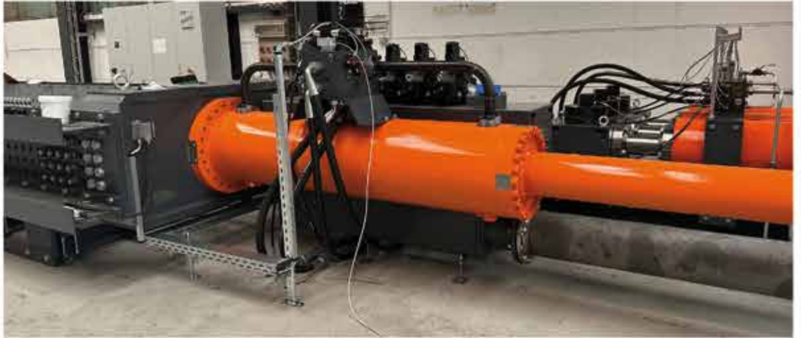
Power in action: the massive hydraulic actuator controls the precise movements. Its size enables the incredible forces and precise reactions necessary for large test systems or demanding load simulations.
