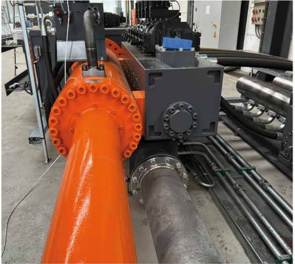
The valve station and the massive valve block. The hydraulic flow is directed precisely via this central unit according to the respective requirements, such as increasing and relieving pressure or dynamic load changes.
