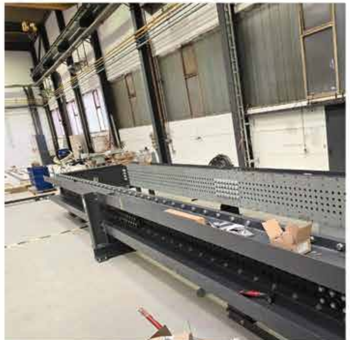
The huge testing frame acts as a rigid structure for applying large forces and movements during component testing. It forms a stable counterforce to the actuators and enables precise load scenarios under realistic conditions – a central requirement for quality assurance in testing.
