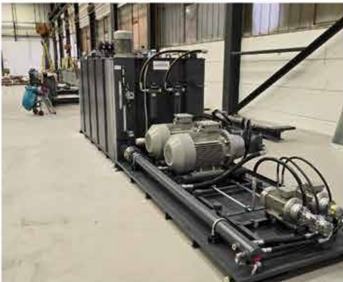
The hydraulic unit. The pump units, filters and sheathed piping can all be seen clearly. The entire system is designed for maximum performance and reliability, with a high output and precise pressure control for demanding testing processes.
