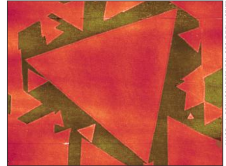
These materials are made from molybdenum disulfide, a two-dimensional semiconductor, grown on a sapphire surface. The triangular shapes seen are aligned because of a special process called epitaxy, where the material follows the pattern of the surface it's grown on. Insulating layers, like amorphous boron nitride, are added during the process of making these ultra-thin materials, which are used to build next-generation electronic devices.
