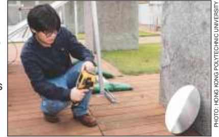
The environmentally friendly SARC coating can reduce a building's surface temperature by up to 25°C and lower indoor temperatures by 2 to 3°C, without consuming any energy.
