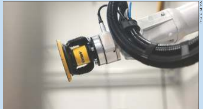
The Mirka AutoChanger is a smart robotized solution for reliably changing abrasives in an automated process, making it much easier to operate robotic sanding systems.
