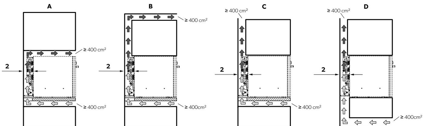
2\* : Minimum 15 mm distance between the minibar's back (incl. the cooling unit) and the surrounding structure)
