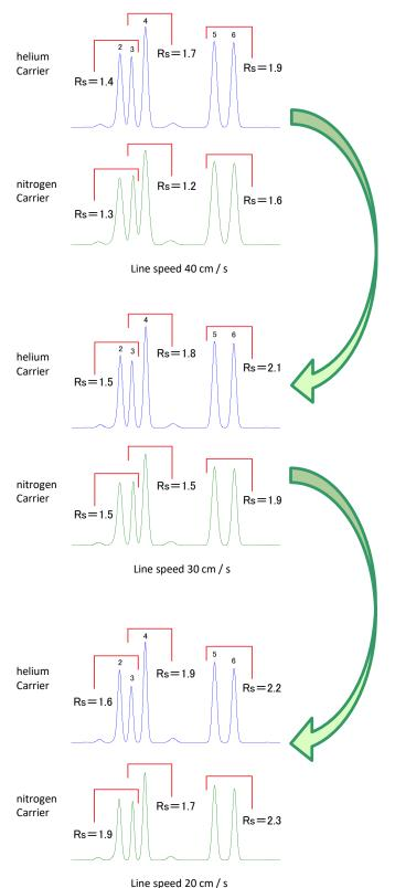
When the carrier gas is changed from helium to nitrogen, it can be seen that the peak resolution after changing the carrier gas visually decreases at linear velocities around 40 cm/s. When changing the carrier gas, compare the degree of peak separation under the analysis conditions in which the linear velocity is set to be gradually decreased as shown below.
