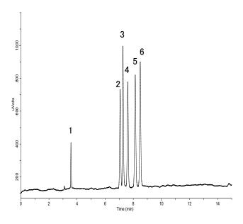
**Conditions** GC4000 Plus type-A(DSTF) System : Column: InertCap WAX  $0.32 \text{ mmI.D.} \times 60 \text{ m df} = 1.0 \,\mu\text{m}$ 65 °C Col.Temp.: Carrier Gas: He 3 mL/min TCD 100 mA(Temp.: 120°C) Detector: Det.Gain: Low split 1:10(Temp.: 200 °C) Injection : Sample Size: 1 μL
