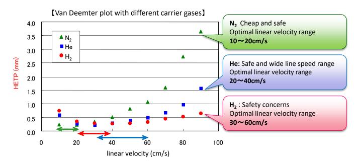
When changing the carrier gas, sufficient separation may not be obtained if the original conditions are applied as they are. In such a case, perform analysis in the optimum linear velocity range of the carrier gas to be used.
