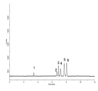
Conditions Carrier Gas: N<sub>2</sub> 3 mL/min Detector: TCD 60 mA(Temp.:120°C) \* Other conditions are the same as for He carrier analysis.
