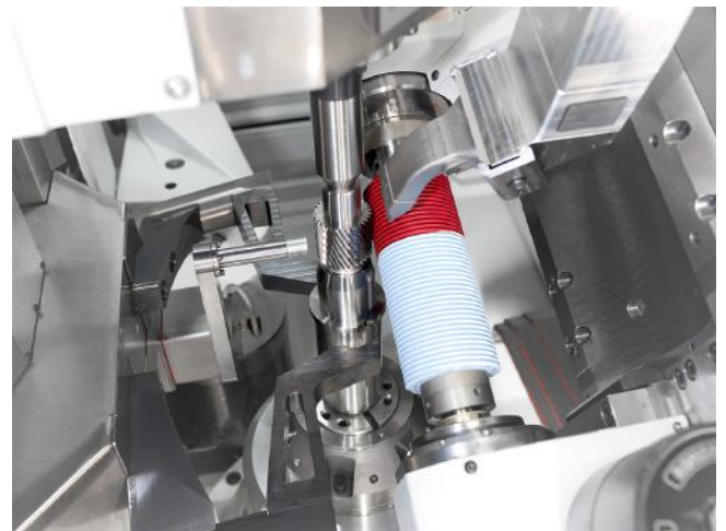
Fig 2: Grinding of an e-mobility shaft with a combined grinding worm
