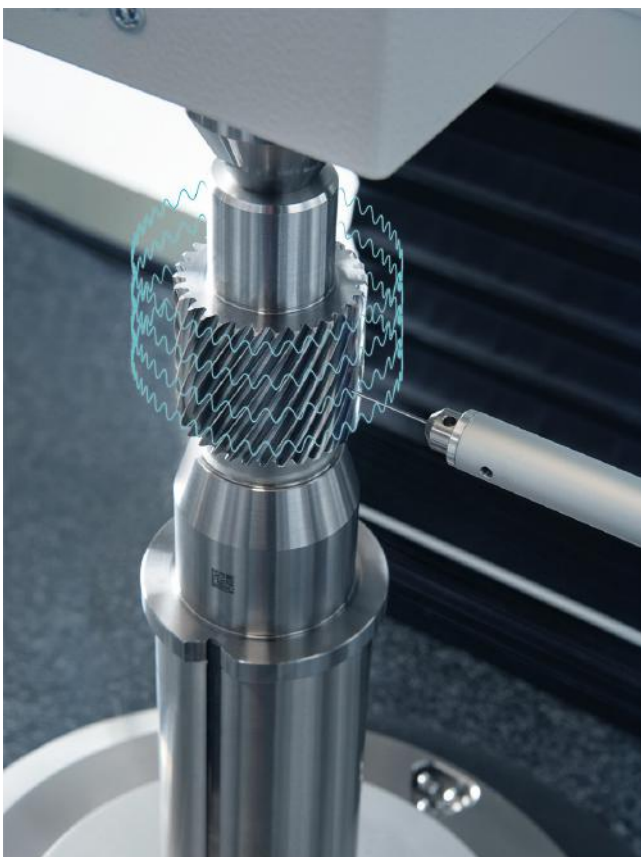
Fig 4: Process monitoring during the measuring of an e-mobility shaft
