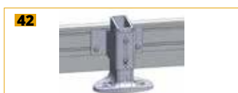
42 Toe board anchor for railing, flat and on plain steel deck Height 150 mm WV841001
