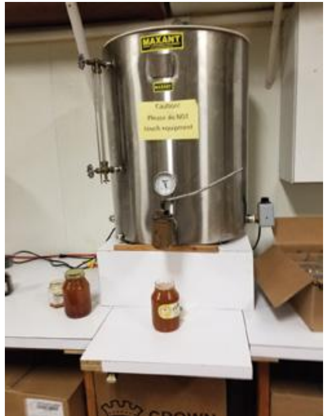
A water jacket botler. Note the elevated stand to allow easy bottling.
