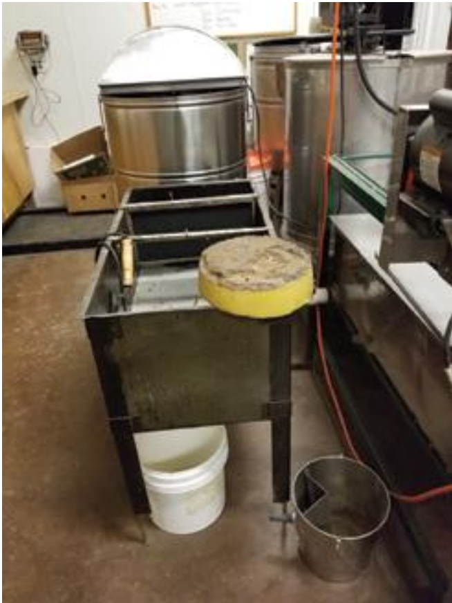
Uncapping tank to uncap frames into and to hold uncapped frames prior to transferring to extractor. Note the beeswax cake with slum gum on bottom (turned upside down).
