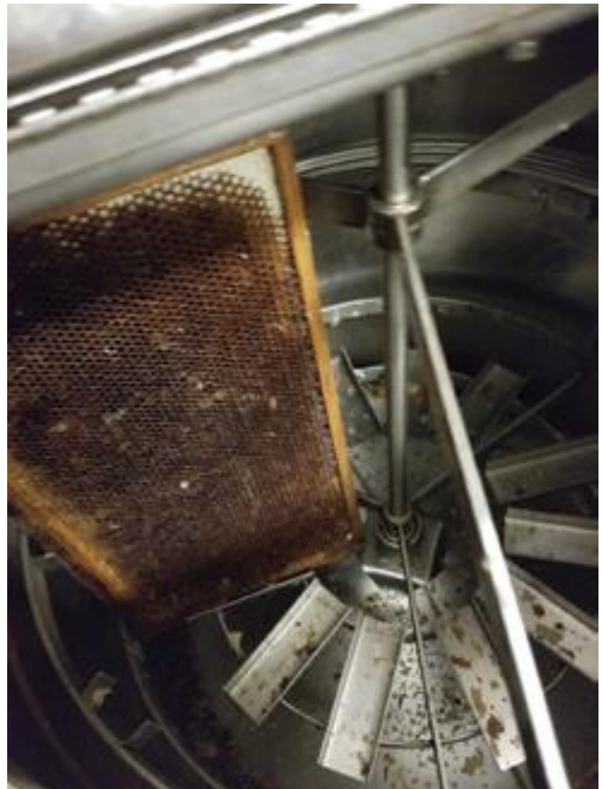
Inside a radial extractor with a brood frame inside for show.
