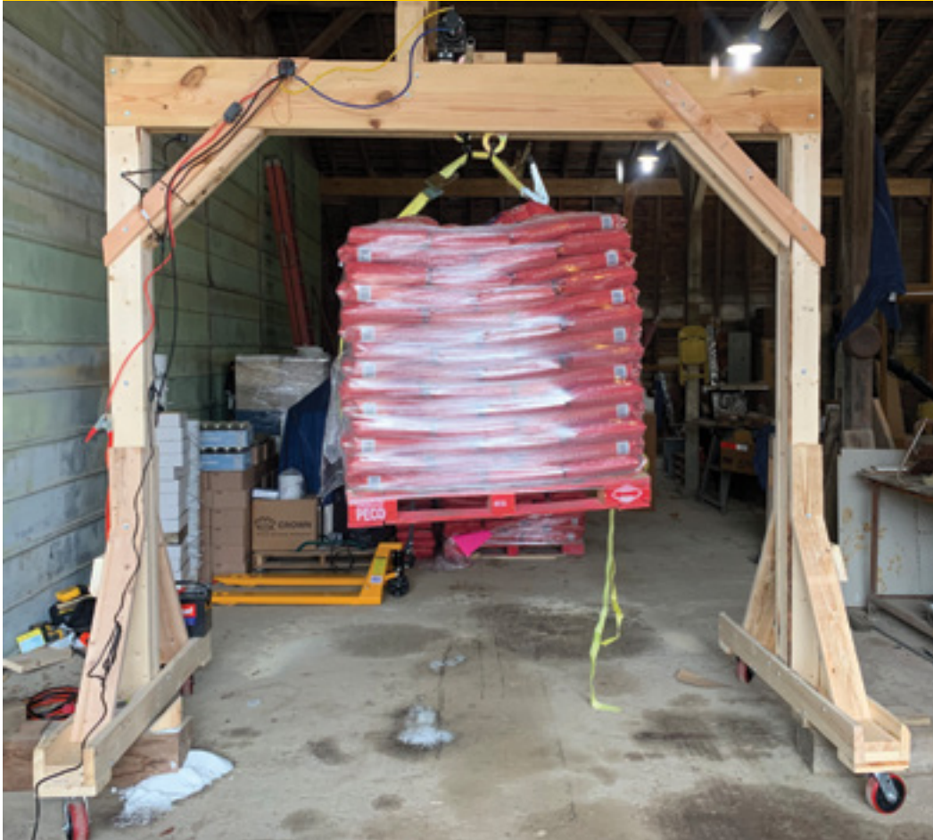
Picture 2. My home-made gantry crane and a 2400-pound pallet of sugar. This will be used to get heavy pallets off my truck and onto the floor where I can move them with a pallet jack.
