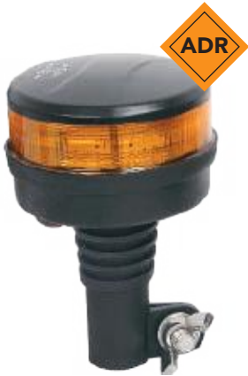
LED BEACON LIGHT AMBER Pole mounting, 12-30V, IP67, ADR approved, ECE R65 10 light patterns, Ø 92mm, height 139mm Art. 5809051 € 65,00 excl. VAT / € 78,65 incl. VAT
