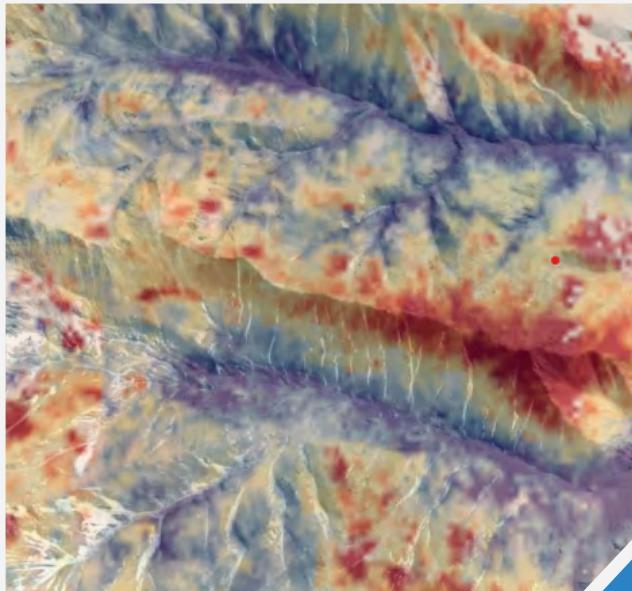
Interferometry is a technique that uses two or more SAR (Synthetic Aperture Radar) satellite images to measure ground displacement with high precision.
