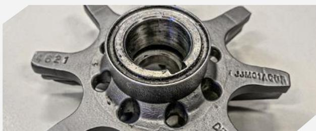
Based on the base material of the impeller, we define the parameters and printing strategy necessary to obtain a stable microstructure, reliable mechanical properties, and metallurgical compatibility during deposition. The process integra-
