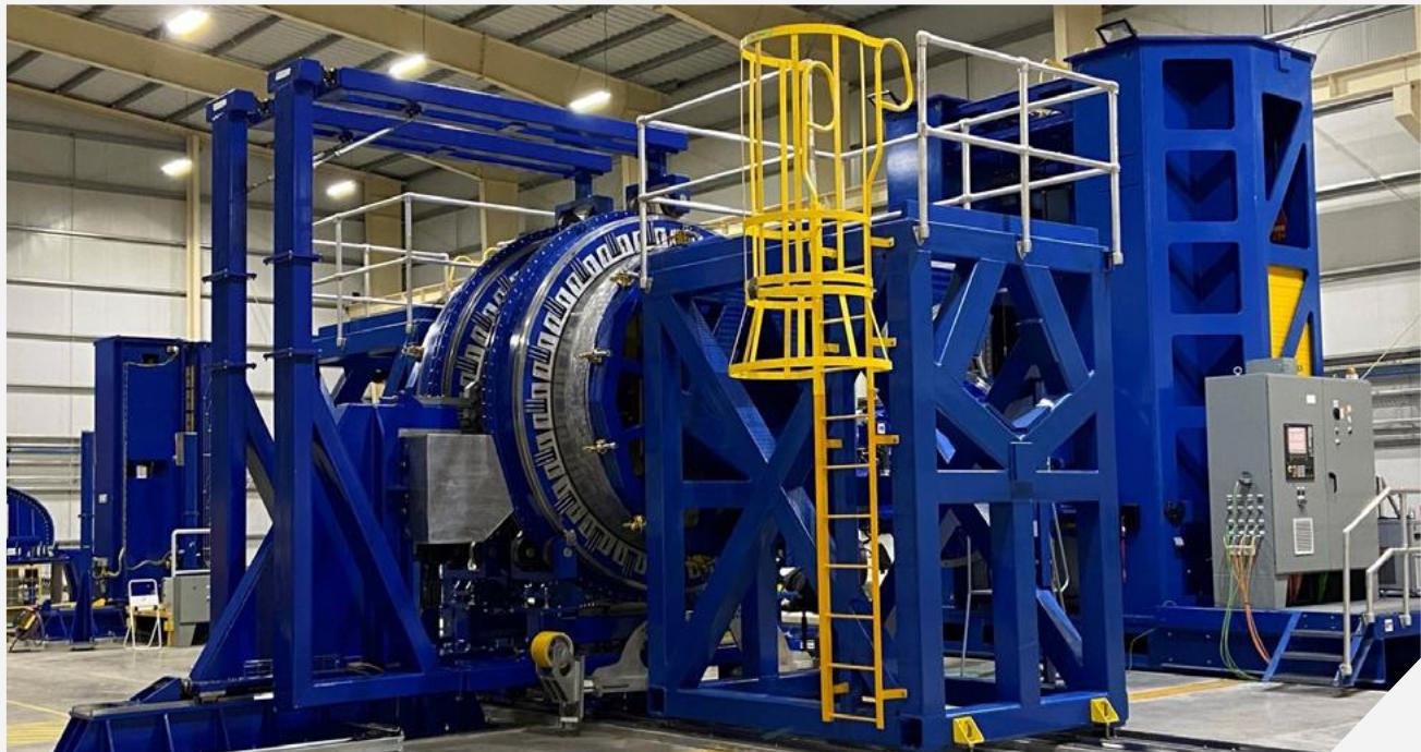
**A solid-state welding process that uses a non-consumable tool to join two pieces without melting their material.** This allows for very high joint efficiencies in alloys where conventional welding (fusion) degrades mechanical properties by a high percentage. For this reason, friction welding is widely used in the aerospace, naval, and military industries to weld mainly aluminum alloys.
