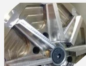
With this methodology, we are able to repair the part with minimal distortion—on the order of tenths of a millimeter—and reproduce the blades in Inconel 718, a material that provides a substantial improvement in wear resistance. This type of application extends the service life of the impeller, optimizes maintenance times, and reduces costs associated with the complete replacement of critical components, consolidating additive manufacturing as a strategic tool for the energy industry.
