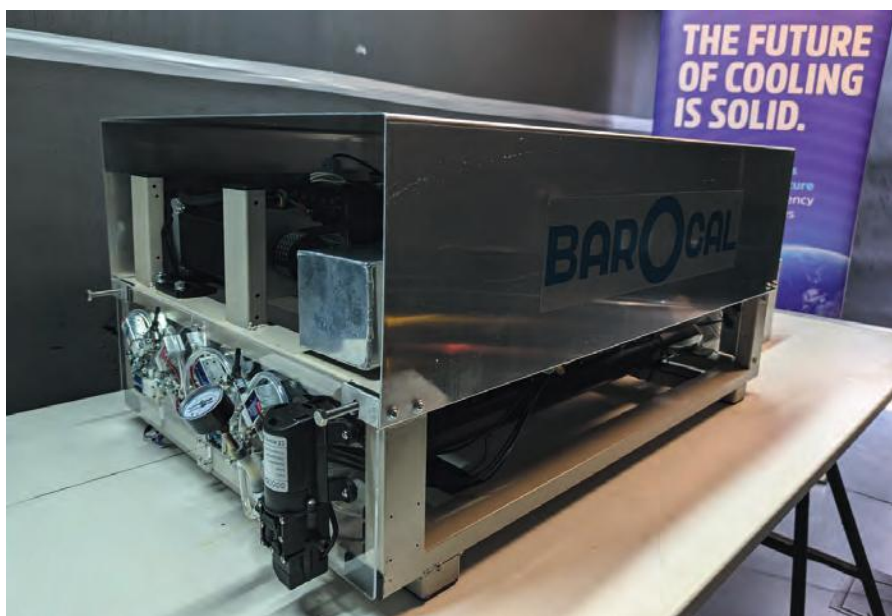
Barocal's latest TRL5 prototype is said to deliver cooling powers and temperature spans in line with vapour-compression systems while surpassing them in terms of energy efficiency
