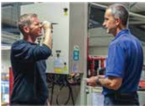
Testing the coolant with a refractometer
