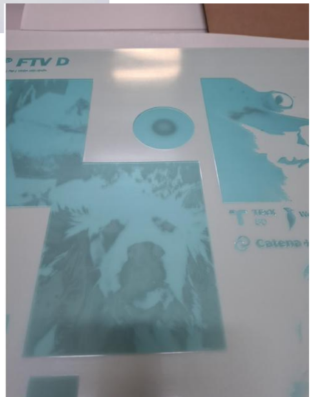
nyloflex® FTV with AIF Directly after stopping the press without any cleaning intervention
