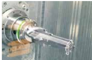
A PCD-tipped high-volume milling cutter from the SPM range
