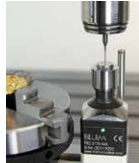
Z-PICO – Tool Setting probe for drilling bit breakage detection and length measurement in micro-machining
