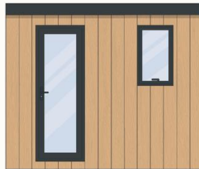
UPVC single door fully glazed left opening 600m wide by 1m high casement window
