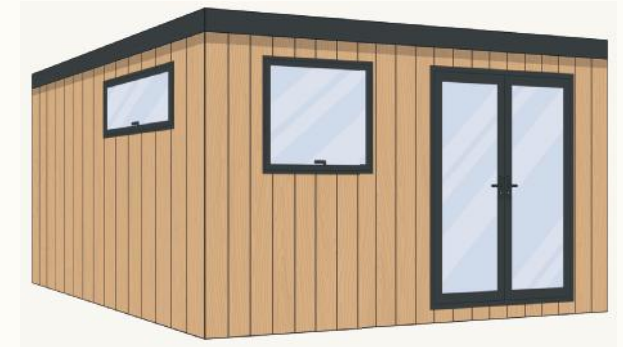
1.8m French doors 1.2m wide by 1m high casement window 1m wide by 600mm high casement window
