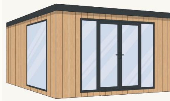
1.8m UPVC French doors with 600mm side windows 1.2m wide full length left picture window
