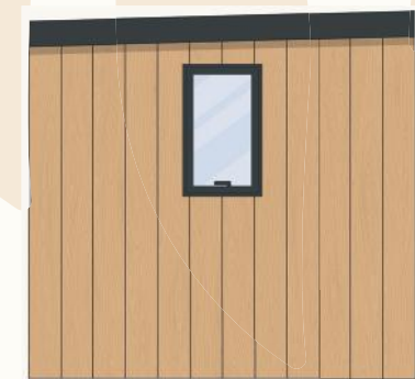
600m wide by 1m high casement window
