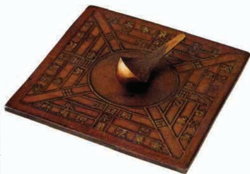
FIGURE 1.2 The first magnetic compass was probably made in China during the Qin dynasty, 200 BCE and used for early navigation.
