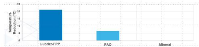
Fig 8: Lubrizol OGLs with PP technology shows better performance in temperature reduction in FZG rig
