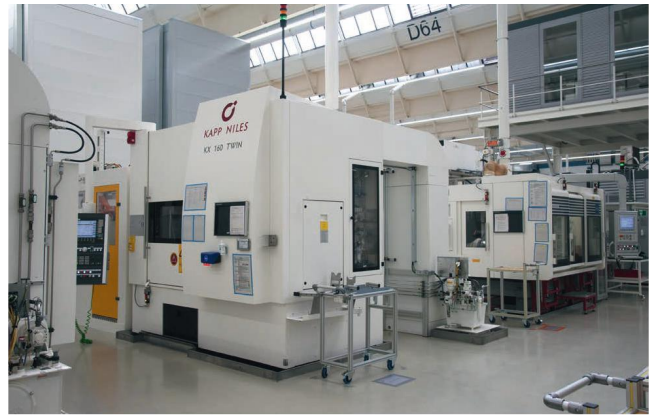
Figure 3: In shaft production: The KX 160 TWIN © Martin Witzsch same size. Thus, he has to changeover the machine, but not the clamping tools. The remaining set-up time is minimised by the intelligent set-up concept of the KX 100 DYNAMIC. For one machine, he needs just 20-25 minutes.
