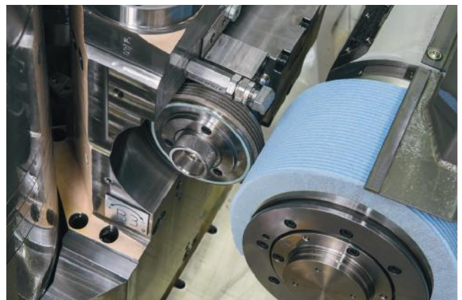
Figure 4: With a 5-pass full profile roll, the dressing time can be reduced by more than half without compromising on quality © KAPP NILES
