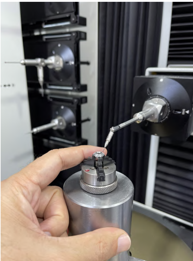
0.5 module gear measurement on Gleason 475 GMS
