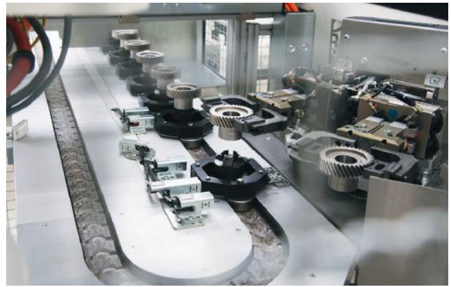
Figure 6: Loading to and unloading from the conveyor belt is done by a transfer unit © Martin Witzsch
