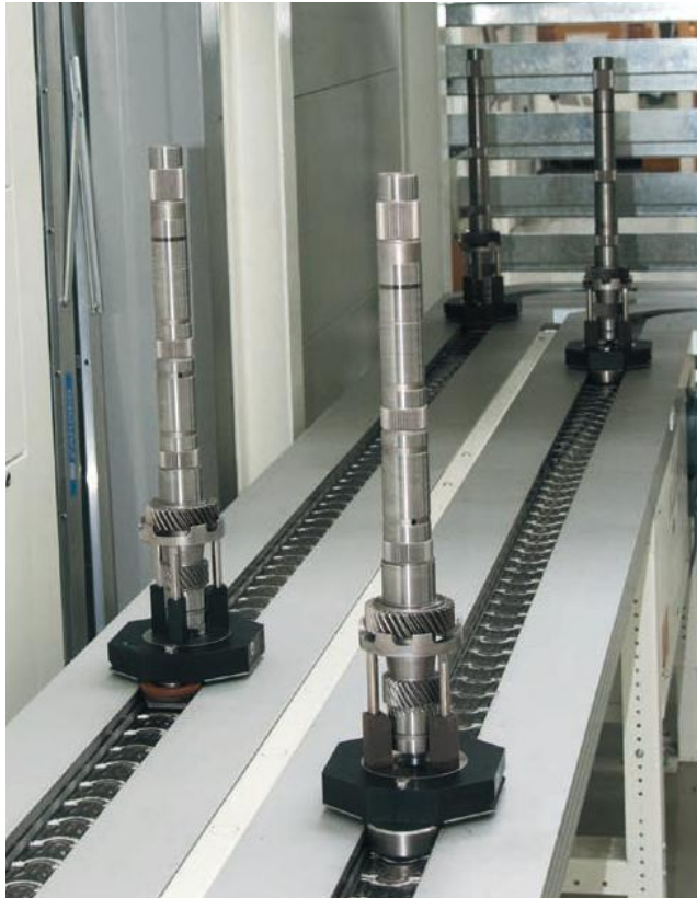
Figure 7: The long shafts are hollow and thus comparatively unstable, making the grinding process particularly challenging © Martin Witzsch
