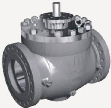
When maintenance in line is required, top-entry ball valves are available. With the stem in the vertical position this valve design permits disassembly, replacement of the all internal parts and seals and reassembly without removing the valve from the line.
