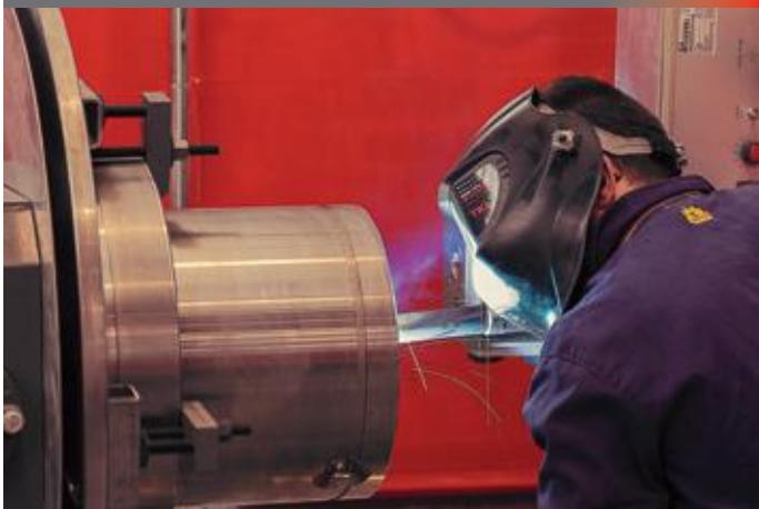
JC Valves provides the best welding technology for any kind of welding needs. Weld Overlay is a welding process, offered on request, where one or more metals with specific characteristics are applied to a base metal to improve desirable properties or to restore the original dimension of the components that significantly enhances the service life of them.
