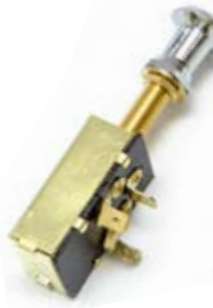
MP39590** MP39592 (Bulk 100pcs./carton) OFF-ON(1)-ON(1&2) SPDT • First pull energizes #1 • Second pull energizes both circuits • Solid brass construction • 3/8" mounting bushing • 3 blade terminals • For panels up to 1" thick • Chrome finish plastic knob • Rated: 15 amp @ 12 VDC
