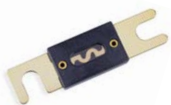
Available with various AMP ratings at 32VDC. Ceramic Body for Superior Insulation Brass, Gold-Plated Element for Superior Electrical Contact Ignition Protected (ISO8846)
