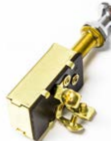
MP39640 MP39642 (Bulk 100pcs./carton) OFF-ON(1)-ON(2) SPDT • First pull energizes #1 • Second pull energizes circuit 2 • Solid brass construction • 3/8" mounting bushing • 3 screw terminals • For panels up to 1" thick • Chrome plated solid brass knob • Rated: 15 amp @ 12 VDC
