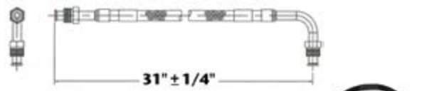
18-8114 FUEL LINE HOSE UNIVERSAL For fuel pump to carburetor connection. Replaces copper or steel tubing 3/8" X 31" PTFE composite hose with 5/8"-18 male inverted flare straight one end, 5/8"-18 90° one end. SAE J1527 type A1
