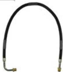
18-8115 FUEL LINE HOSE UNIVERSAL For fuel pump to carburetor connection. Replaces copper or steel tubing 3/8" X 25" PTFE composite hose with 5/8"-18 male inverted flare straight one end, 5/8"-18 90° one end. SAE J1527 type A1
