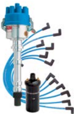
18-26002-1 IGNITION SYSTEM KIT Fits: GM 4.3L/262 CID Even Fire Engines
