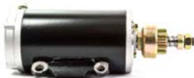
18-5634 OUTBOARD STARTER Replaces: 585057, 585051, 385529, 389954, 586283 Fits: 140 HP models (1977)
