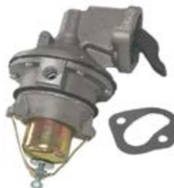
18-7278 FUEL PUMP Flange I.D. # M60032 Replaces: 86234A4, 86234A05, 86234A3, 86234, 77594, 71327, 47585 For: GM (4 & 6 Cyl.) 153, 181, 225, 250, 120 / 140 / 160 / 165 / 470 / 485 / 488 Uses filter 18-7860 & gasket 18-0889
