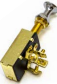
MP39622 (Bulk 100pcs./carton) OFF-ON(1)-ON(2&3) SPDT • First pull energizes #1 • Second pull energizes two separate circuits • For anchor/running lights or similar function • Solid brass construction • 3/8" mounting bushing • 4 screw terminals • For panels up to 1" thick • Chrome plated solid brass knob • Rated: 15 amp @ 12 VDC
