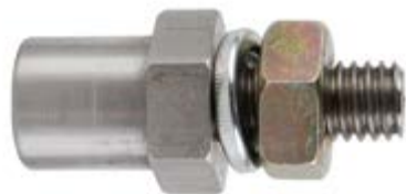
18-8412 STARTER STUD EXTENDER Extends the solenoid stud on PMGR starters for applications that require more accessory wire connections. Threads: Female M8x1.25, Male 3/8" x 16 UNC
