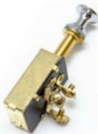
MP39580** MP39582 (Bulk 100pcs./carton) OFF-ON(1)-ON(1&2) SPDT • First pull energizes #1 • Second pull energizes both circuits • Solid brass construction • 3/8" mounting bushing • 3 screw terminals • For panels up to 1" thick • Chrome plated solid brass knob • Rated: 15 amp @ 12 VDC
