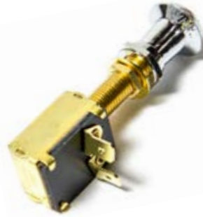
MP39530** MP39532 (Bulk 100pcs/carton) OFF-ON SPST • Pull for ON • Solid brass construction • 3/8" mounting bushing • 2 screw terminals • For panels up to 1" thick • Chrome plated solid brass knob • Rated: 15 amp @ 12 VDC
