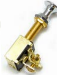
MP39600 MP39602(Bulk 100pcs./carton) OFF-ON (1 & 2) SPST • Pull for ON - turns on two separate circuits • Solid brass construction • 3/8" mounting bushing • 3 screw terminals • For panels up to 1" thick • Chrome plated solid brass knob • Rated: 15 amp @ 12 VDC
