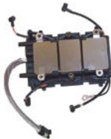
18-5887 POWER PACK Replaces: 584985 For: V6 engines with optical sensor and GRAY sleeve on power pack. Do not use with black sleeved stator.
