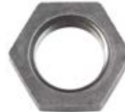
18-3719 PINION NUT Replaces: 11-35921, 11-47411, 11-826375, 11-F694188 5/8" - 18 thread • 1 1/16" wrench
