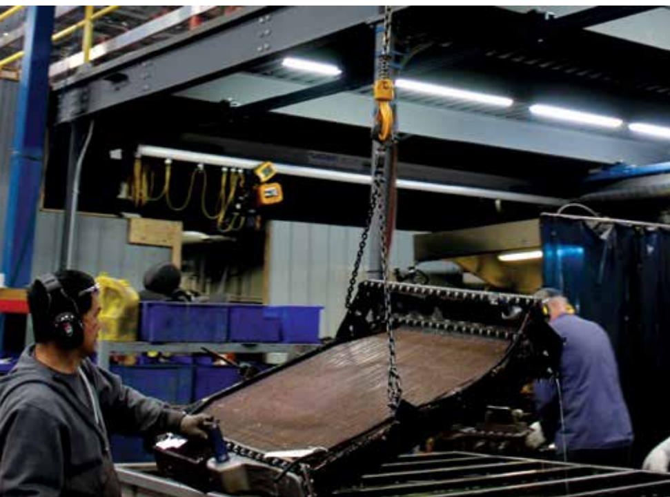
A West End Radiators technician uses an overhead crane to pressure test a frame of the Mesabi rad to ensure it has no leaks.
