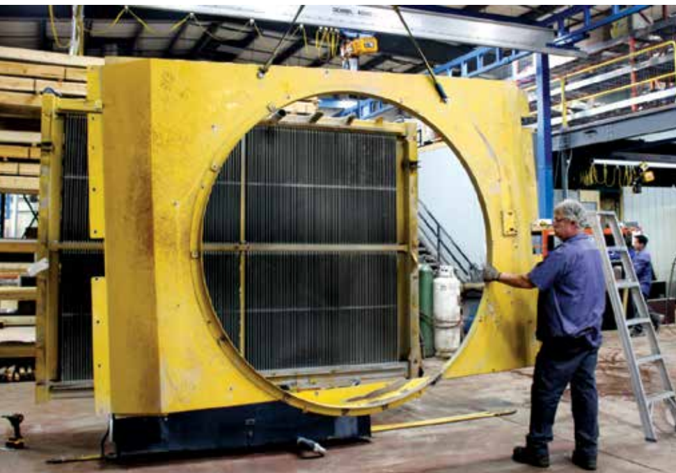
A West End Radiators technician uses an overhead crane to repair a Mesabi radiator.
