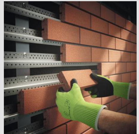
Above: The slips mechanically fix to a steel single-rail system to create a lightweight, A1-rated rainscreen facade that is suitable for mixed-use, mid- and high-rise developments and retrofit applications.
