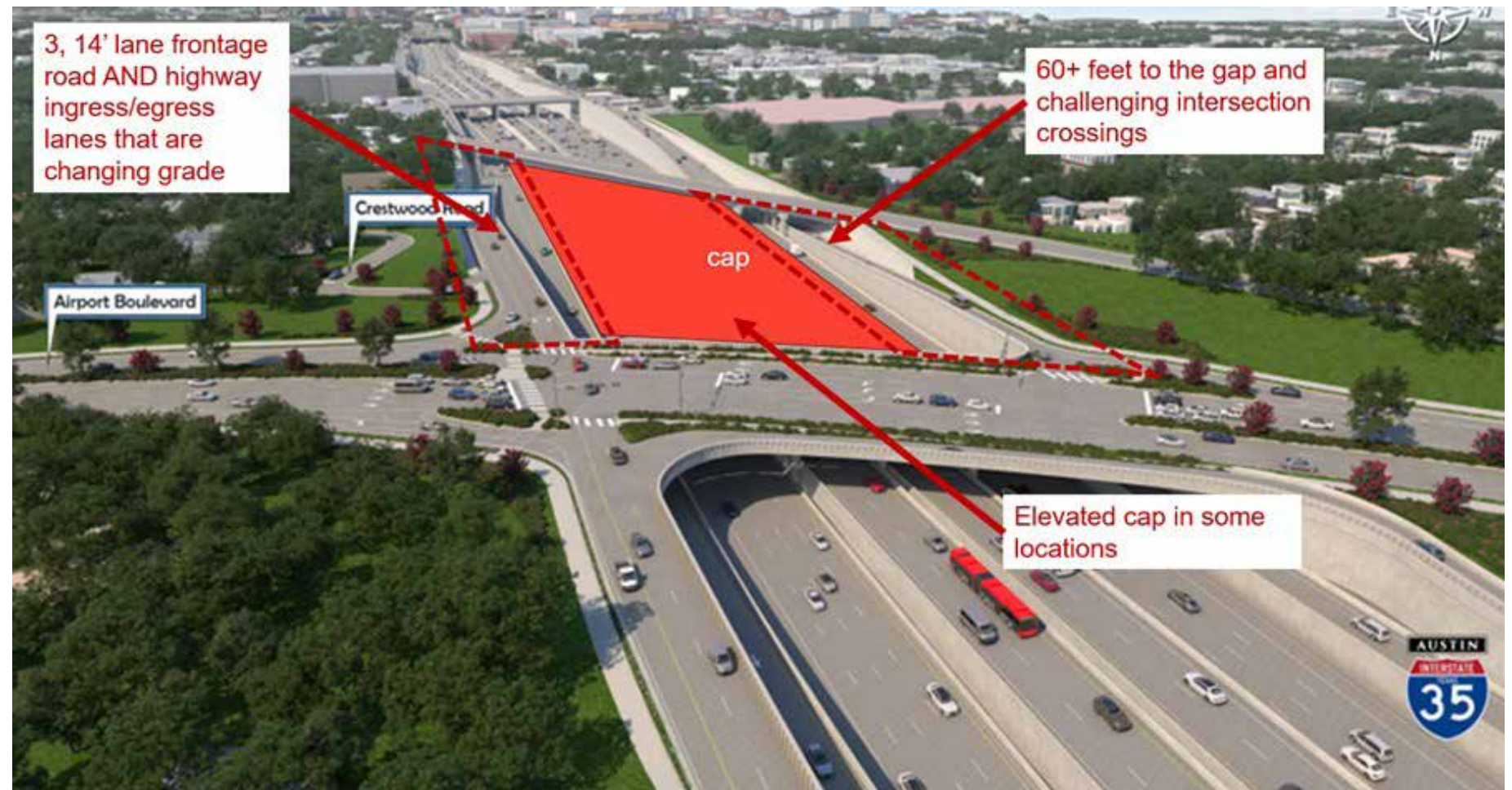
Diagram of the Highway Cap proposed prior to the Spring 2025 City Council vote, and the only originally proposed cap that had a marginal value.
