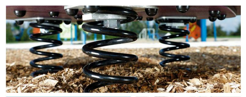
Three coil springs developed specifically for Jambette by a major Canadian manufacturer provide the rocking motion of Equilibra. They are pinch-free for hands and feet. The top end of each spring is fastened to the underside of the equipment platform, while the bottom end is secured to the underground anchoring system by simple design mounting brackets that stand the test of time.
