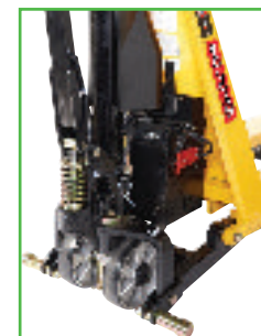
Stabilising bars prevent the unit moving whilst in use
