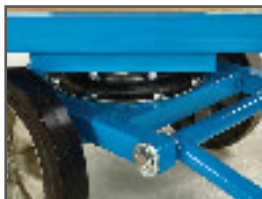
Heavy duty ball bearing turntable assembly for easy movement when fully loaded
