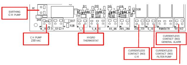
Closes when the unit breaks down Can be applied in a domotic system to indicate a failure
