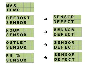
Alarm messages are only messages of an active action which stops by itself or that an action should be taken in order to solve a problem – see <u>ALARM MESSAGES</u>..
