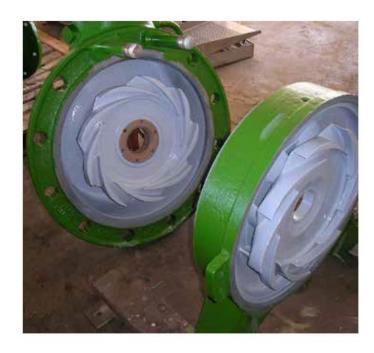
Belzona 1341 (Supermetalglide) is a two-component coating system designed to improve the efficiency of fluid handling equipment and to protect metals from the effects of erosion-corrosion.
