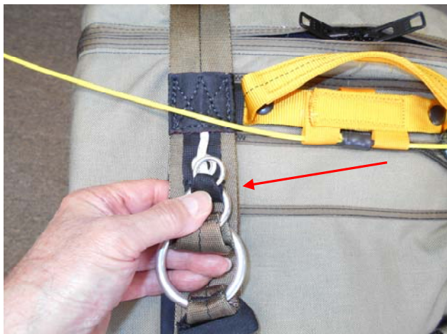
Pass the small Ring of the Riser through the large Ring of the Riser.
