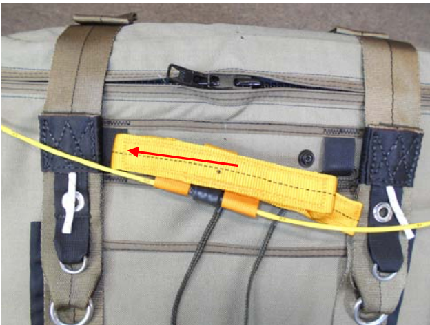
Tuck one tab under the T-4 keeper.
