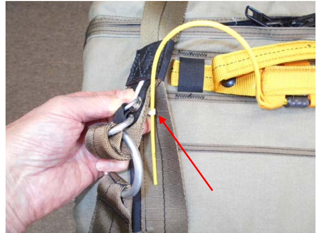
Pass the closing loop down through the top small grommet.
