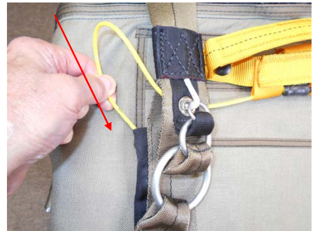
Secure the yellow cable in the black sleeve on the side of the Riser.
