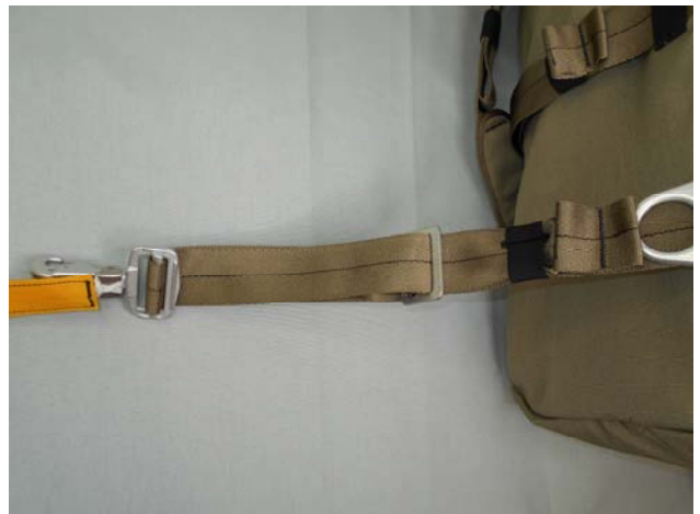
Stow that excess under the Elastic Keeper.
