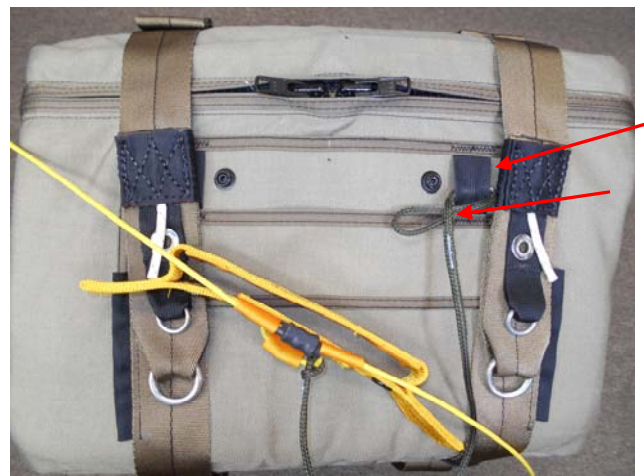
Pass the large Loop of the Safety Lanyard under either of the T-4 keepers shown.
