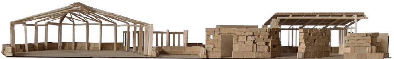
Made at 1:100 Structural Model for a crematorium design
