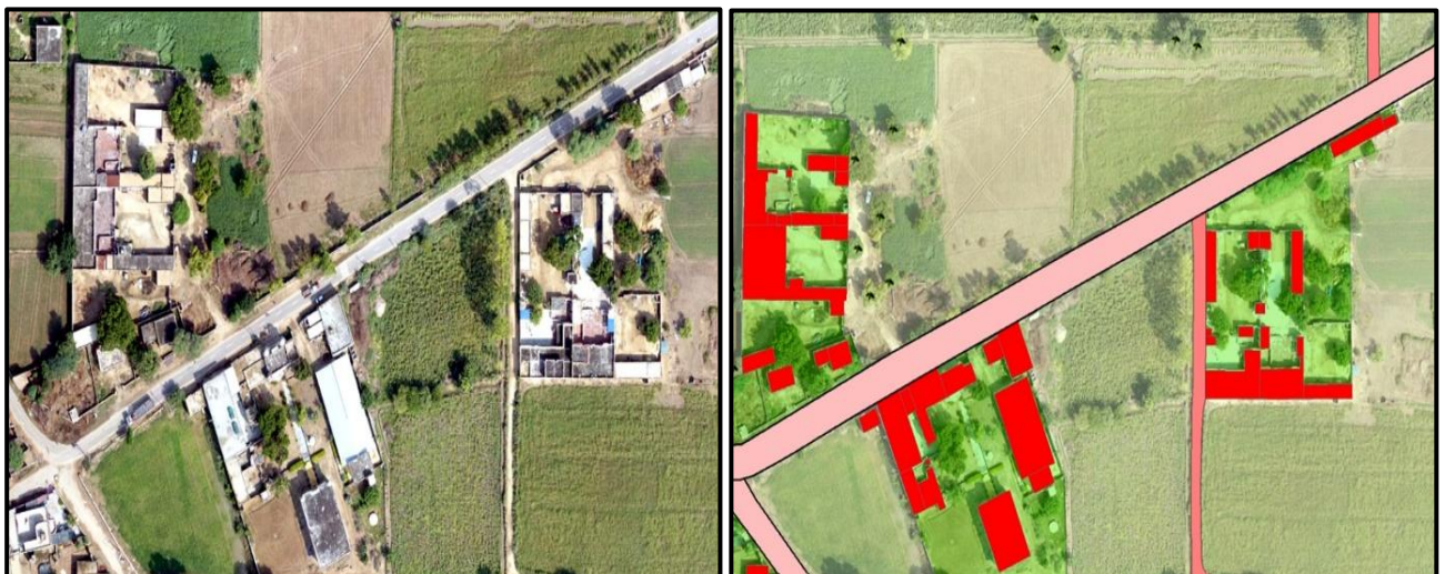
Fig 7: Ortho Rectified Image and feature extraction
