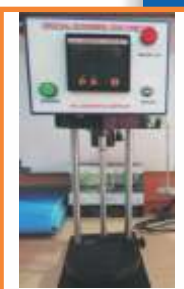
VISCOSITY ASTM D 562
