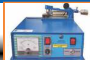
SCRATCH HARDNESS ASTM D 2197, D 7027, BS 3900
