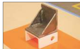
Figure 8: Structural adhesive, Belzona 7311, used to bond bracket.
