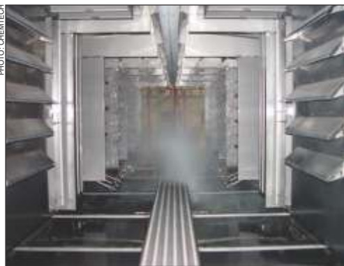
Chemtec's solutions for the treatment of wastewater generated by painting booths using water curtains for overspray separation ensure an extension of the life of the water, reducing disposal costs and ensuring the high quality of the painting process.
