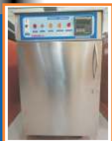
HUMIDITY TESTER ASTM D 2247, ISO 6270
