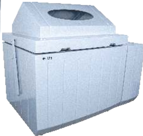
Salt Spray Chamber FRP
