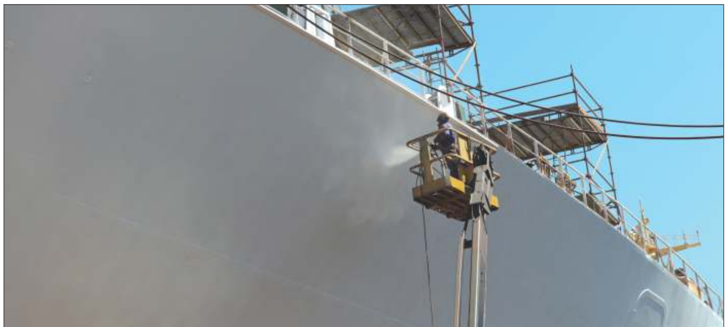
Proper application includes suitable surface preparation, selection of proper primer, intermediate and top coat which can give high durability in a chosen environment.
