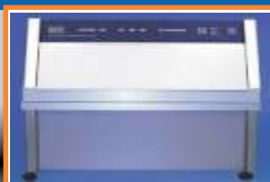
ACCELERATED WEATHEROMETER (QUV) ASTM G 154, ISO 16474
