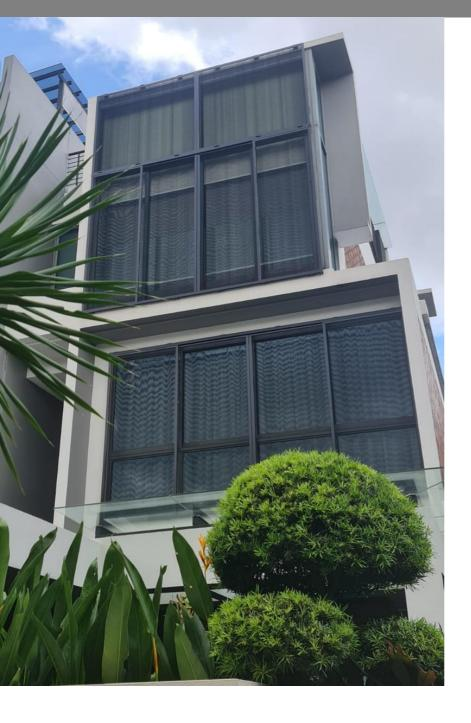
In order for glare to be eliminated, the screens were installed outside, on the roof top terrace as the primary protection.
