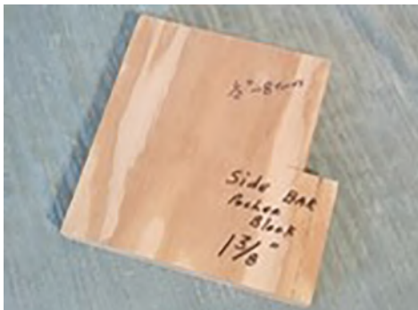
Finished notching jig
