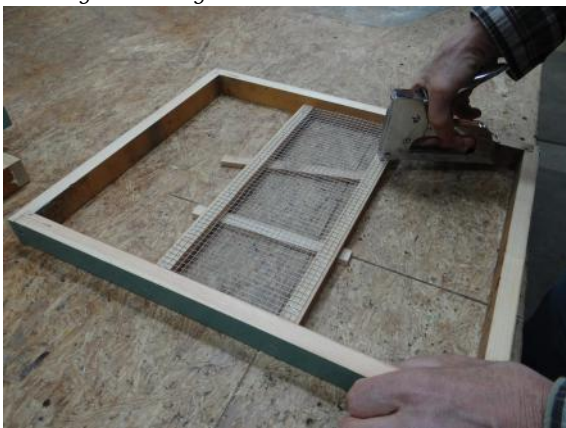
Note the spacers under cross members, raising them ¼ inch Photo by Eric Talley
