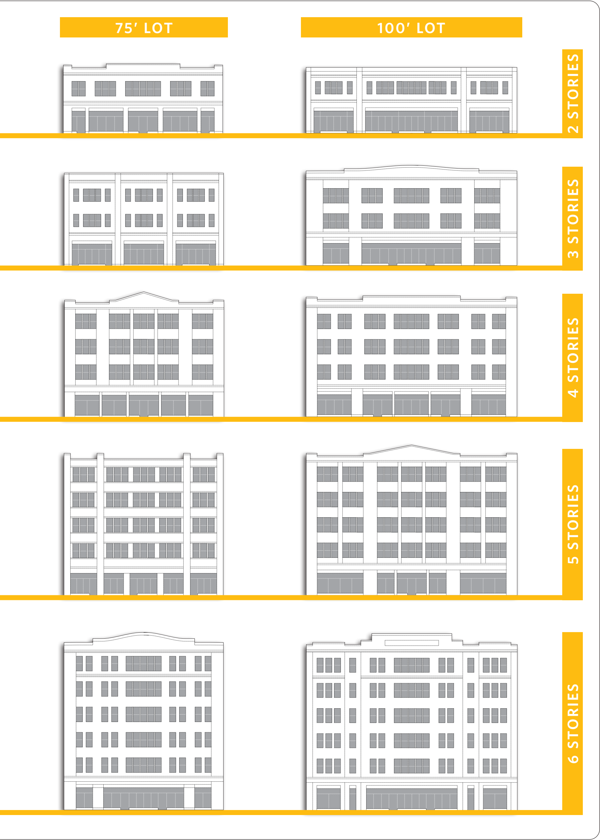
FIGURE 104: Fabric Building Matrix This matrix represents possible combinations of essential elements of a fabric building. The variety of combinations all feel part of a common language.
