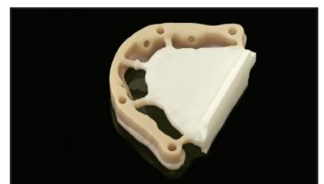
Fig. C The framework is colored and fired while still connected to a piece of the block.
