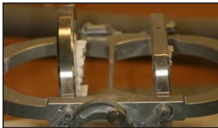
Fig. H The Eco milling machine can be set to different angles to mill every corner of the restoration.
