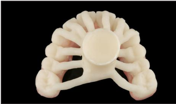
Fig. L Each tooth is connected by its own sprue when the white porcelain layer is pressed.
