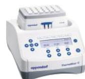
Thermoblocks with Thermal cap and adapters for 0.5mL and 1.5mL tubes, deep well 500 plates, 96 and 384-well PCR plates.
