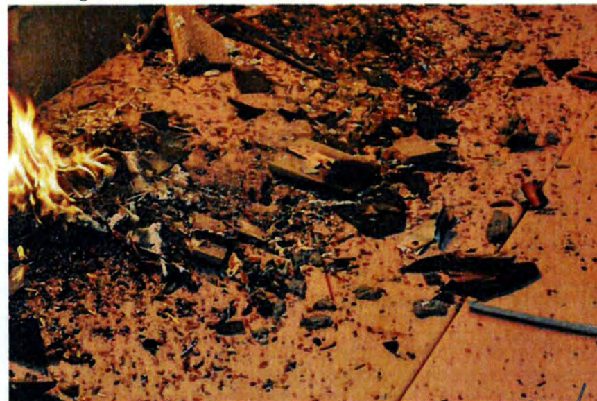
Fig. 34. View of the test element which had fallen off by the 17 th minute of test
