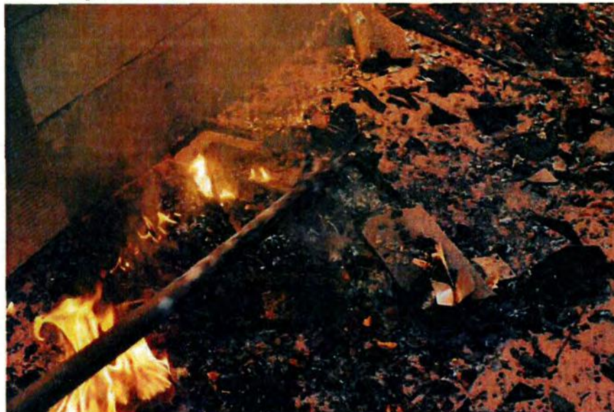
Fig. 36. View of elements which had fallen off before the 26 th minute of test
