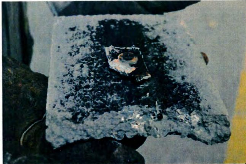
Fig. 26. View of elements which fell off in the 5 th minute of test
