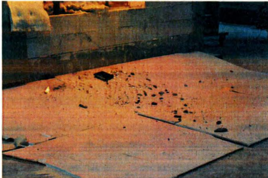
Fig. 24. Fragments which fell off in the 4 th minute of test
