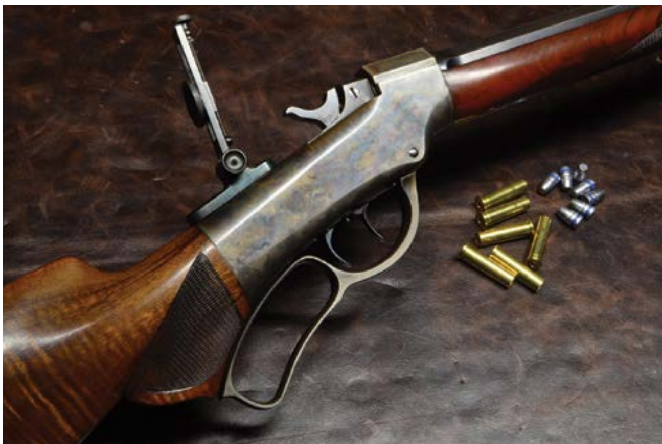
Ballard Union Hill No. 8, manufactured by Marlin in the 1880s, chambered in .32-20 and fitted with a mid-range tang sight and globe (non-adjustable) front sight. For a "moderately priced" target rifle, this one is certainly striking.
