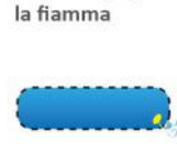
The air coming out from the hole extinguish the flame itself
