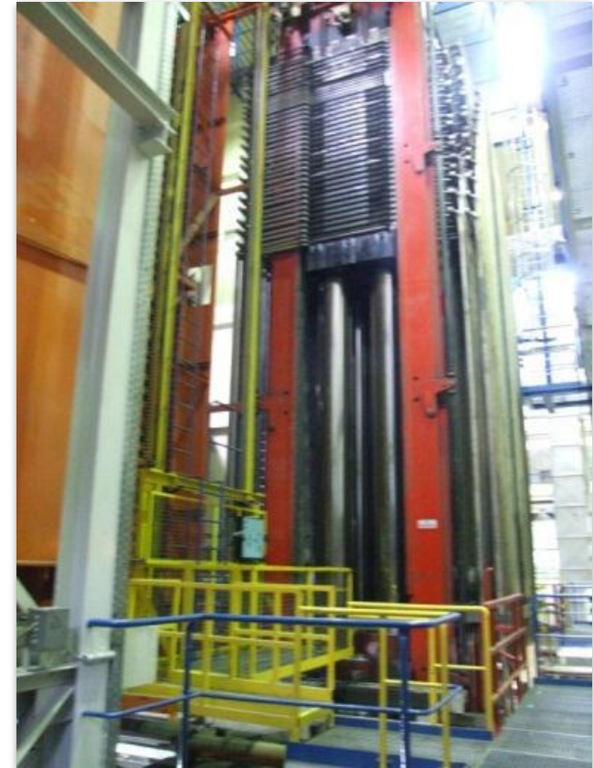
44 daylight press Largest stationary HPL press in the world
