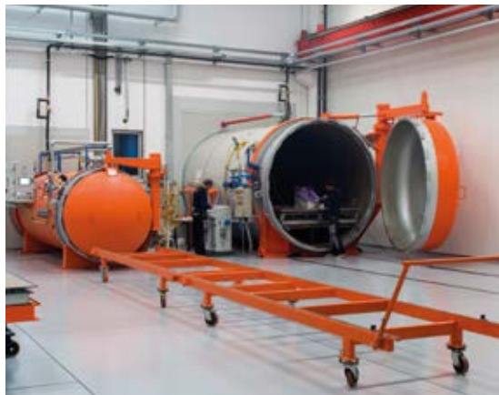
Autoclaves for parts provide up to six atmospheres of pressure ensuring full laminate consolidation.
