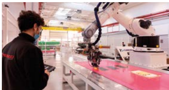
Automated tape laying robot 'Lola' at work.
