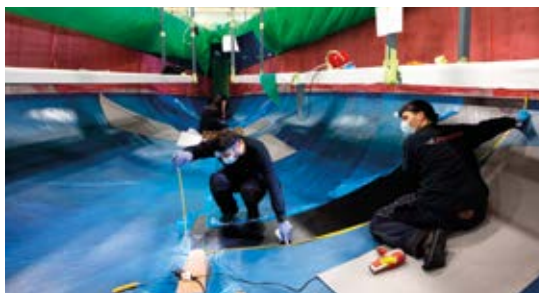
Prepeg carbon hull creation.
