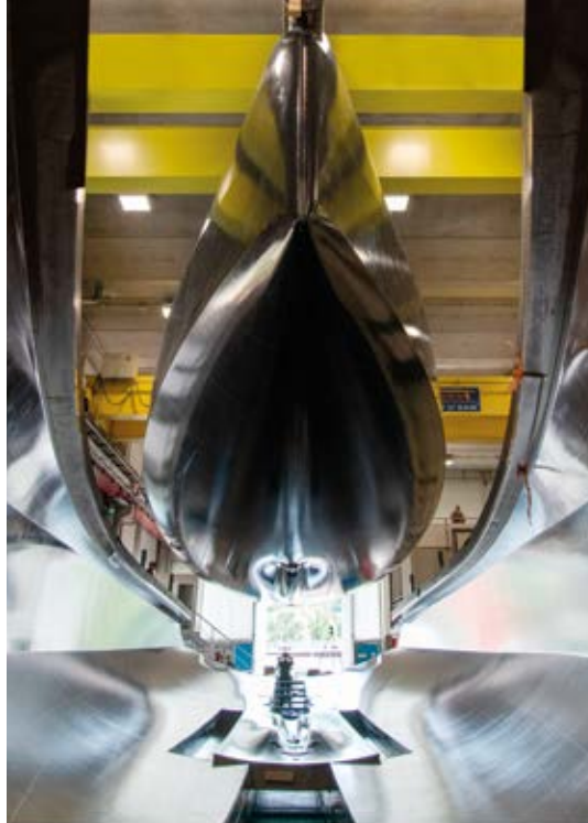
Demoulding from precision in-house tooling.
