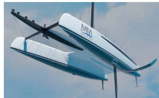
Showing her six foil configuration, including her rake-able righting moment foils.
