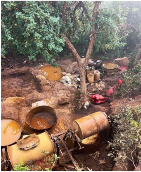
Basic gold mining tools used by zama zamas near Pilgrim's Rest, including sluice boxes, pans, and hand-operated equipment, which contribute to riverbank disturbance and sedimentation in the Blyde River catchment.
