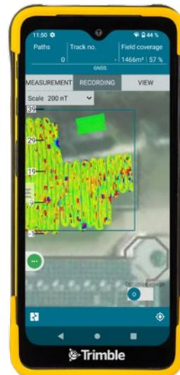
Data acquisition of freely customizable field configurations as well as direct magnetic field display in color, also with GNSS (exemplary screenshot with VFC4.2)
