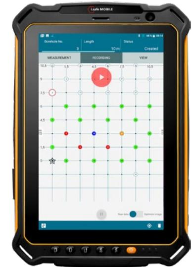
Convenient data acquisition and navigation in the borehole field (exemplary screenshot with VFC4.1plus)
