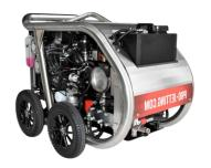
Petrol High Pressure Pro Cart Power (kW) 30 | Power (HP) 40,8| Pressure (bar) 300 | Pressure (psi) 4350 | Flow pump (LPM) 31,2 | (GPM) 8,3 | Engine / Motor Vanguard 61G2 | Type pump CH 31/300
